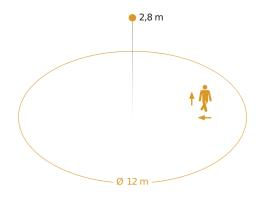
Possible mounting height: 2,50 m - 4,00 m Orange: radial and tangential
